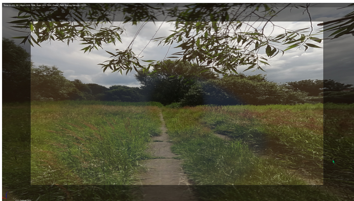
Fig. 18: Image simulation of the torus design with a real photo. The bright area marks the FOV of a 24 mm equiv. photo lens (appr. 70^{\circ} \times 40^{\circ} )
