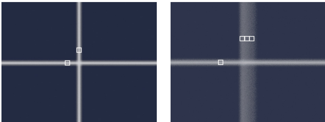
Fig. 15: Beam spread of the coaxial spherical display at center (left) and with the eye camera turned right 20° around the pupil position, assessing the eye peripheral resolution (right). Squares of 1arcmin x 1arcmin are overlaid for comparison. The grid lines displayed are originally <1arcmin wide.
